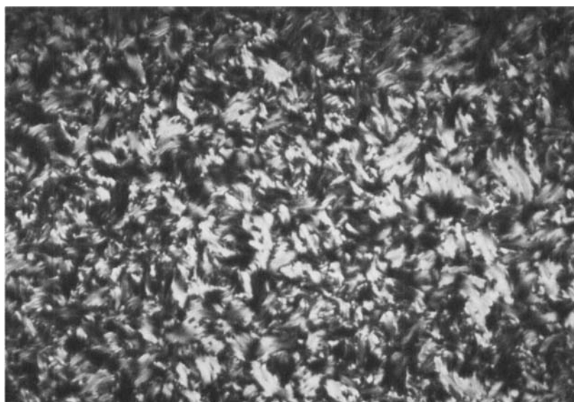
FIGURE 13 Distorted S_A fan texture at Ch-S_A transition in the thioester 4e ( R = C_{10}H_{21} ).
